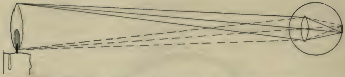
FIG. 80. How an image is formed on the retina of the eye.
